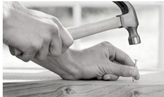
*Hit the Nail:* When using the hammer, make sure to hit the surface of the nail squarely with just the right amount of force. That means not to use all your force to pound hard, nor it be too soft to almost seems like you are just tapping it. And while keeping a good grip, use the distribution of strength of your whole arm and not just solely work on your wrist and hand. In order to hit the nail directly, allow the weight of the hammer to do the work and not your arm.
