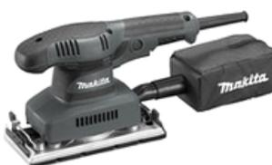
*Sheet sanders* are generally a good deal less powerful than Random orbital sanders and are best used for providing that finishing touch - the final preparation step before applying paint, finish, lacquer, stain, or whatever else. Because of the square shape of the pad, sheet sanders are much more appropriate to use than where you must get right to the edge of 90-degree angles.
